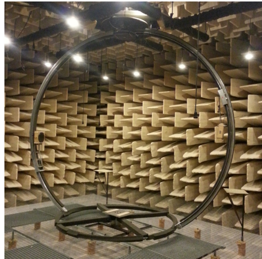
Figure 1: The TASP system in the anechoic chamber of the University of Oldenburg. Note the offset sled mounts, allowing for greater coverage for the vertical positioning of the transducers.
