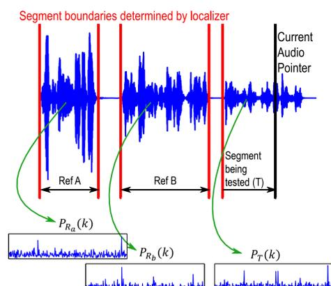
Speech is processed in short time frames (20 ms), with a frame advance of 10 ms. Each frame of speech is converted into Mel-Frequency Cepstral Coefficients (MFCCs), which are the feature vectors.
